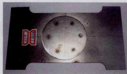
图6 破孔点焊修补试件 Fig.6 Spot welding repair specimen for broken hole
